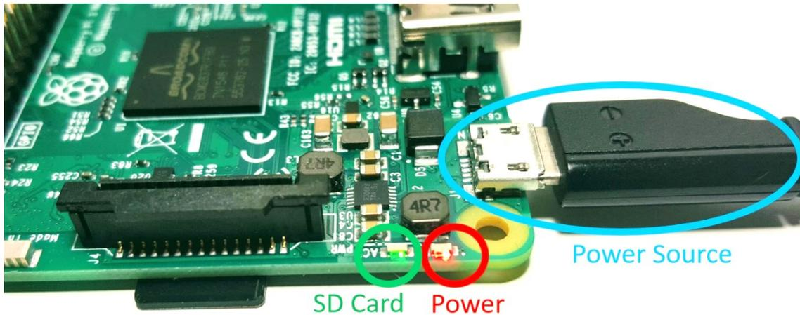
**NOTE: The red Power LED must be always on. If the Power LED is blinking, or is off, the power source from the PSU is not providing enough power to the board.**
